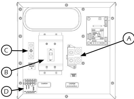
**A. Neutral Lugs**, These neutral lugs are isolated from ground and provided for you to connect your neutral wire from the transfer switch. The lugs on the 60 kW will handle wire sizes #4 AWG to 300 MCM and should be torqued to 250 in lbs. The lugs on the 90 kW will accommodate #1 AWG to 600 MCM and should be torqued to 300 in lbs.
