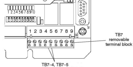
Your DC connection points in the ASCO 185 ATS are terminals "4" and "5" on the interface terminal block. As this is a "DRY" unpowered contact set it set, it makes difference which lead (battery negative #1 or start #23) connect to which terminal.
