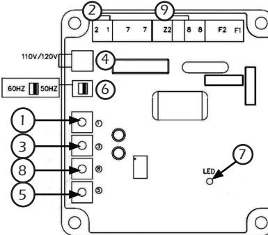
1. VOLTS - Adjust generator output voltage.
