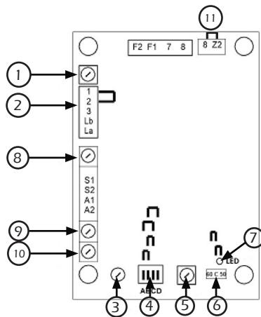
1. VOLTS - Adjust generator output voltage.
